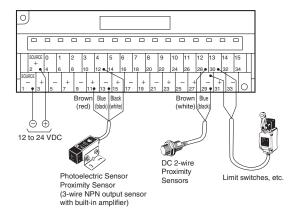
Note: Photoelectric and Proximity Sensor lead wire colors have changed in line with revisions to JIS standards. Former colors are given in parentheses ().
